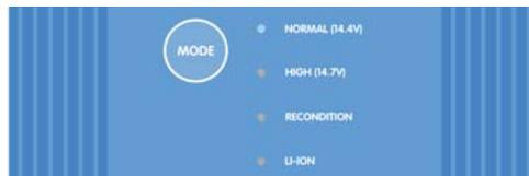
4. If the maximum rated charge current is excessive, enable low current mode (charge current limited to 50% of the maximum rated charge current and disabled fan). To enable (or disable) low current mode depress and hold down the **MODE** button on the **Blue Smart IP22 Charger** for 6 seconds; when enabled the NIGHT LED will blink.
