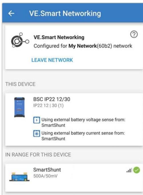
17. For systems with additional VE.Smart networking compatible chargers connected to the same battery / battery bank, repeat steps 8 to 16 above to include each remaining charger into the common VE.Smart network.
