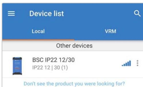
6. **VictronConnect** will attempt to establish a Bluetooth connection with the **Blue Smart IP22 Charger** and display the connection progress in the Connecting pop-up dialog box.
