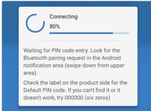
7. When attempting to establish a Bluetooth connection with a new/unpaired device, the Bluetooth pairing request pop-up dialog box will appear after a short delay; enter the default PIN code stated on a label located on the back of the charger (or try 000000 if there is no default PIN code label), then select **Pair**.
