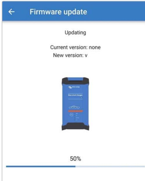
7. If the firmware update does fail for some reason, a notification with the failure reason will be provided within the Firmware update page; select **Continue** to exit into the **VictronConnect** Device list Local page and re-attempt the firmware update.
