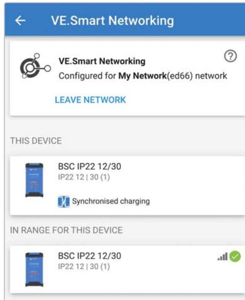
17. For systems with additional VE.Smart networking compatible chargers connected to the same battery / battery bank, repeat steps 9 to 17 to include each remaining charger into the common VE.Smart network.
