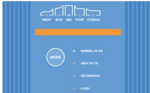
2. Depress and hold down the MODE button on the **Blue Smart IP22 Charger** for 10 seconds.
