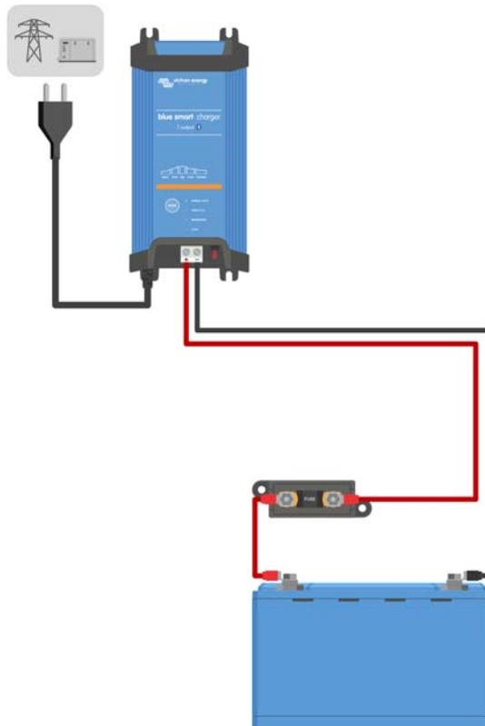
3. Connect the **Blue Smart IP22 Charger** AC power cable to a mains power outlet; after a short delay the LEDs indicating the current charge mode and charge state will illuminate.
