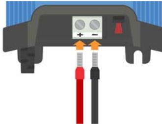
D. Torque the terminal screws to 2.4Nm using a suitable torque wrench and screw driver bit, then reinstall the terminal cover.
