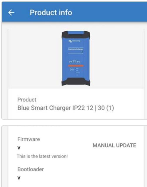
9. Select the **Blue Smart IP22 Charger** firmware file that has just been manually loaded from the the Firmware library page (if multiple firmware versions have been manually loaded, ensure the correct version is selected) to access the Firmware update page.
