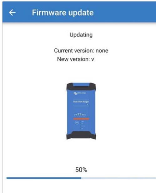
13. If the firmware update does fail for some reason, a notification with the failure reason will be provided within the Firmware update page; select **Continue** to exit into the **VictronConnect** Device list Local page and re-attempt the firmware update.
