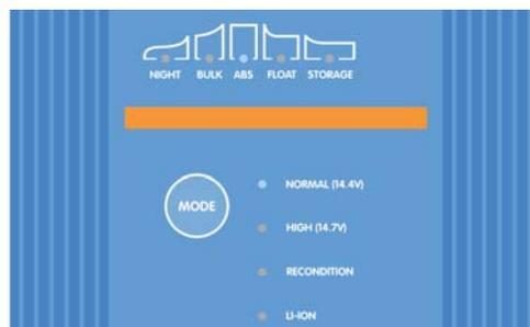
4. Select the charge mode and charge current limit most appropriate for the battery type and capacity.
