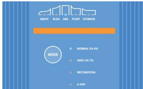
2. Press (and release) the **MODE** button on the **Blue Smart IP22 Charger** to cycle through and select the most appropriate integrated charge mode (Normal, Normal + Recondition, High, High + Recondition or Li-ion).
