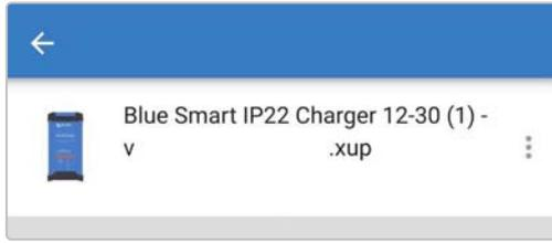
10. If no firmware files are listed within the the Firmware library page, the Firmware file previously loaded is likely not compatible with the specific **Blue Smart IP22 Charger** model or hardware version being updated.
