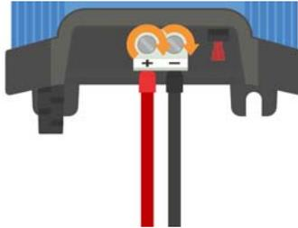
2. Install a suitably rated inline fuse or circuit breaker within the DC power cabling between the **Blue Smart IP22 Charger** and battery/batteries, located as close as practical to the battery/batteries; refer to the 'Installation > Wiring > Overcurrent protection' section for more information.
