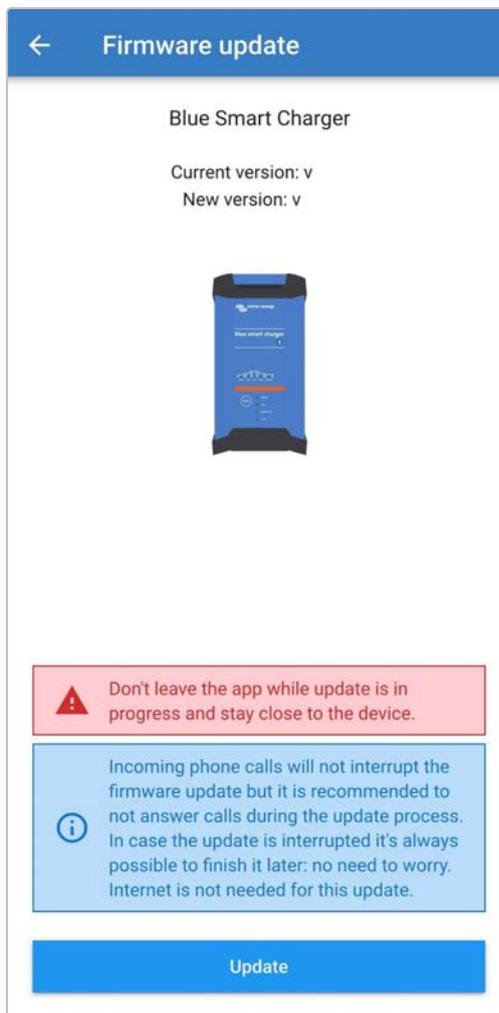
6. The firmware update will commence and a progress bar will be displayed within the Firmware update page. Ensure that the Bluetooth enabled device (mobile phone or tablet) remains close to the **Blue Smart IP22 Charger** until the firmware update is complete and avoid using the device during this period; be patient as the firmware update may take several minutes to complete.
