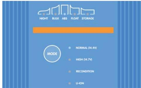
2. Using a Bluetooth enabled device (mobile phone or tablet), open the **VictronConnect** app and locate the first **Blue Smart IP22 Charger** in the Device list Local page, then connect to the device the default PIN code is stated on a label located on the back of the charger, or try 000000 if there is no label).
