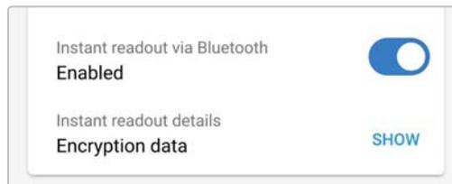
If the instant readout encryption data (MAC address and encryption key) is required, select **SHOW** from the Instant readout details field to open the Instant readout encryption data pop-up dialog; this data is **not** required for normal instant readout functionality via the **VictronConnect** app, it is only relevant for advanced integration of the instant readout data with third party Bluetooth devices and software.
