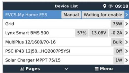
Highlight the EVCS then press spacebar or cursor right to enter the next menu and at the setup menu item press spacebar again to enter the setup menu. See the [EV Charging Station setup \[37\]](#) and the [Description \[2\]](#) chapter for the meaning of the available options.
