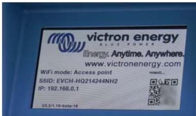
Once connected to the access point, enter the default IP address 192.168.0.1 into a web browser. The default username is "admin". The default password is printed on the sticker inside the unit. The First setup process will then start:
