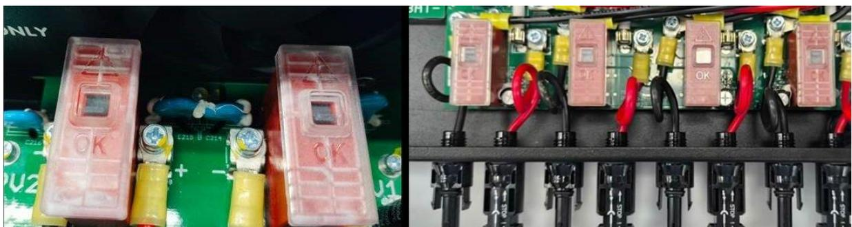
Under normal operating conditions, the small black flag on top of the relay should be in the "OK" position. Additionally, a green LED on the PCB will be lit, indicating that the safety circuits are actively monitoring for hazardous situations.
