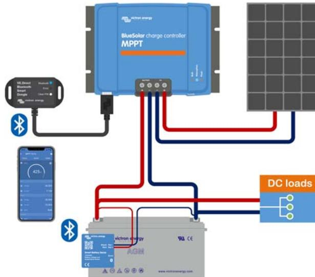
Example of a VE.Smart Network of a Smart Battery Sense and a solar charger.
