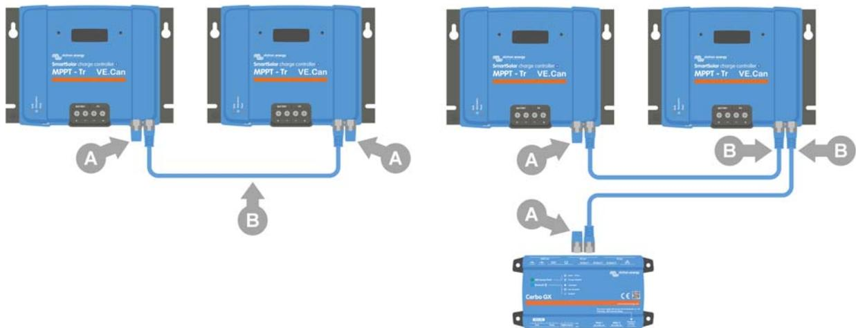
A: VE.Can terminator - B: RJ45 UTP cable.
