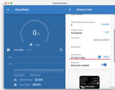
**i** Note that for the SmartSolar VE.Can MPPT 250/100 with a serial number between HQ2150 and HQ2250, the reset procedure – unfortunately – often does not work. In this case, contact your dealer for replacing the solar charger under warranty.
