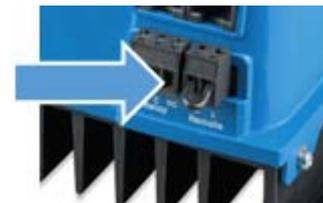
*Remote connector with the wire loop.*
