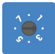
Rotary switch set to position 2
