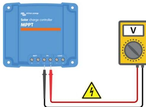
**⚠️ WARNING:** Certain solar charger models may have PV voltages up to 250Vdc. Voltages exceeding 50V are generally considered dangerous. Only a qualified technician should handle dangerous voltages.
