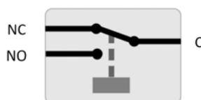
Relay configuration (not energised).
