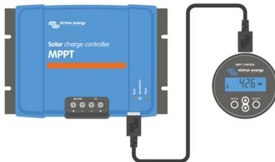
Connect the display to the solar charger via a VE.Direct cable
